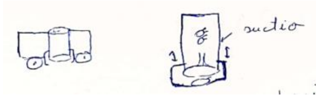
Figure 11: Sketch of Suction Tube with a Gripper
