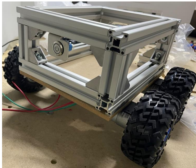
Figure 39: Robot Chassis with Motors and Wheels
