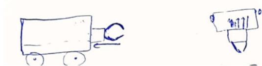
Figure 15: Sketch of Horizontal Gripper
