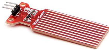
Figure 41- Water Level Sensor Hardware
