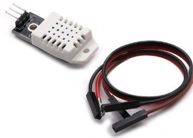
Figure 35- Temperature and Humidity Sensor Hardware
