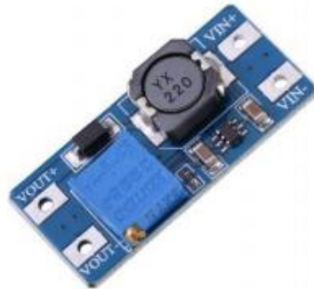
Figure C4: DC to DC Boost Converter.
